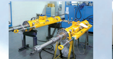
Servomotors (hydraulic hoist) - manufactured & tested by RUHFUS
