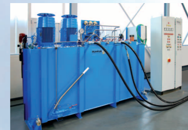
Sample power pack and electrical control panel
